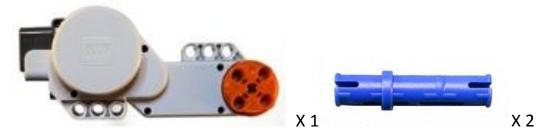
Find one motor and two long blue connectors. Fit them together as shown below. Note that the motor goes *inside* the vertical beams, and the blue connectors protrude inwards.
